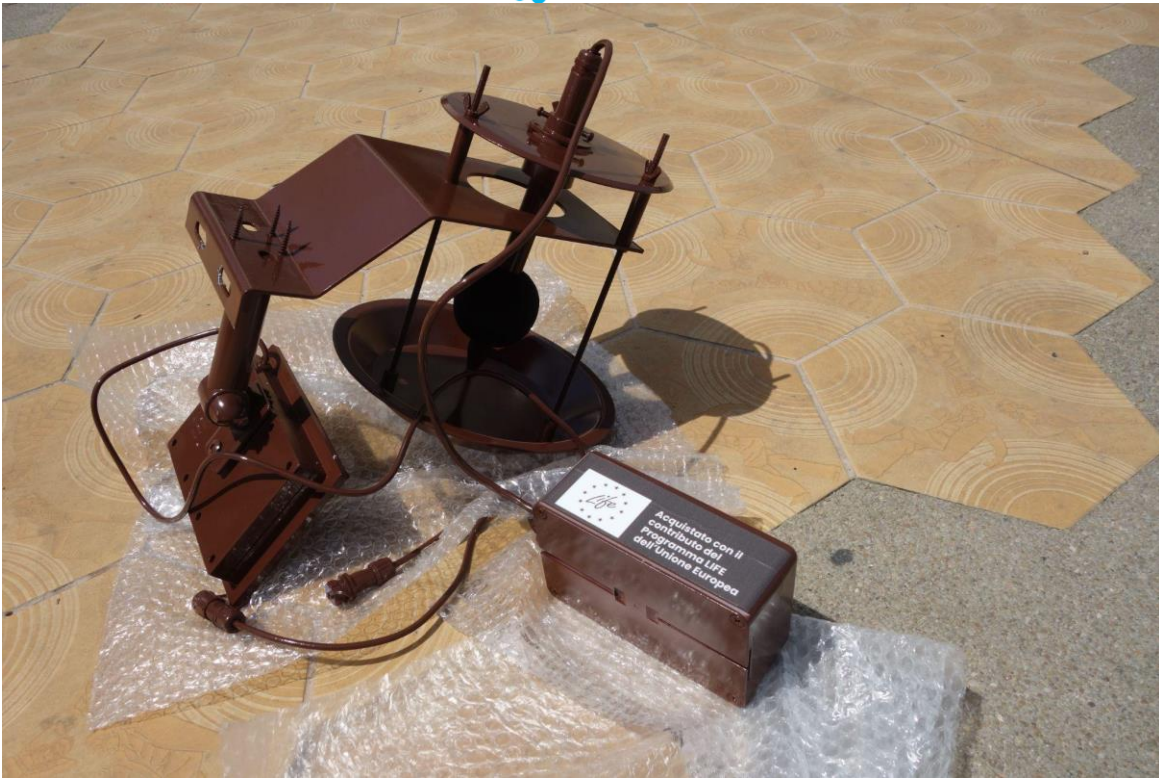
Figure 8: Noise sensor in brown colouring for the streetlights with corten effect painting.
