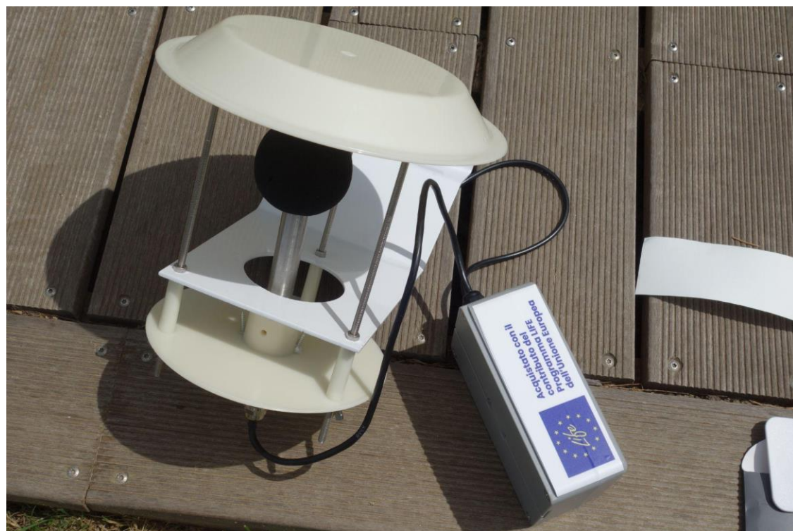
Figure 7: Noise sensor in white colour for the streetlights without any finishing paint, on which the sticker with the references of the European funding and the project logo is also visible.
